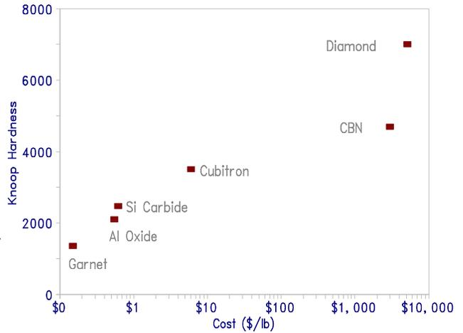
These materials are available in a wide variety of sizes and in several purities. The grain is crushed and passed through sieves to segregate it into common particle or grit sizes, denoted numerically. The larger the number, the smaller the particle. Common sizes run from 16 grit (coarse) to 220 grit (fine). As a rule, the coarser materials are used to make rough cuts for heavy stock removal and the finer grits are used to make delicate cuts in finishing operations.
